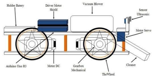
Figure 5. The physical design of the tool side view
