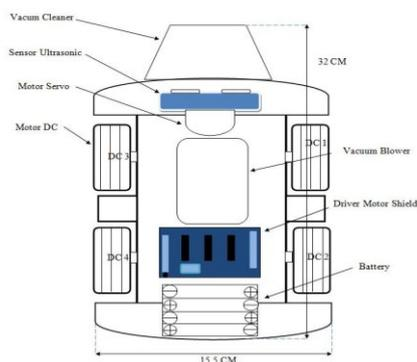
Figure 4. The physical design of the tool, top view
