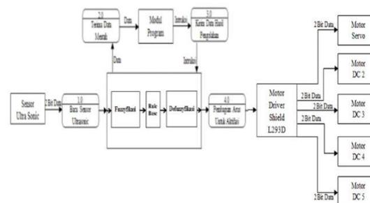
Figure 2. Data Flow Diagram
